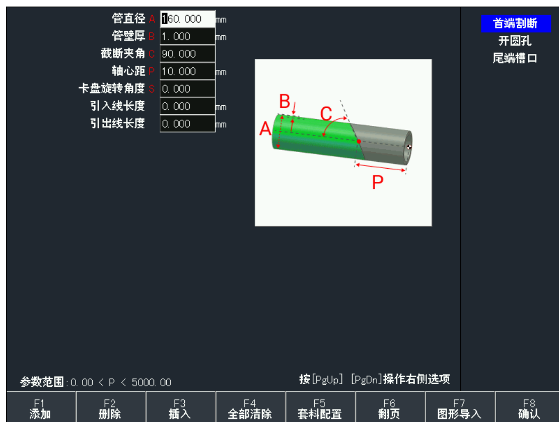
Figure 9.3 Tube cutting element combination and setting parameters
