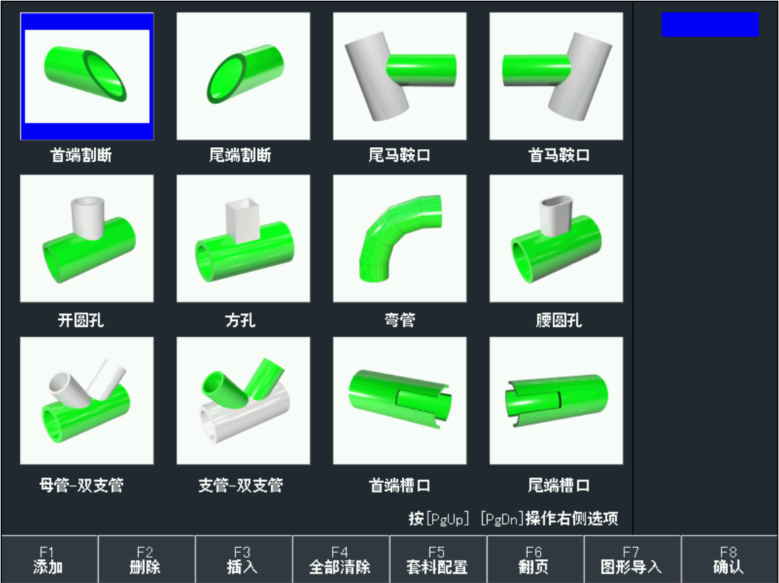
Figure 9.1 Pipe cutting library interface I
