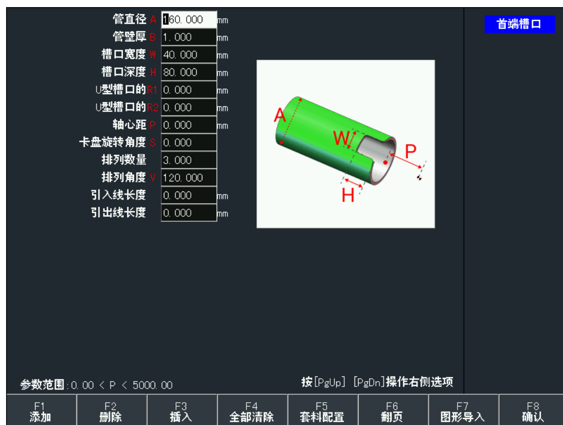
Figure 9.1 Interface for parameters of the 8 terminal slots
