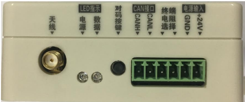
Figure 11.1 Backside interface of receiver 5F1522
