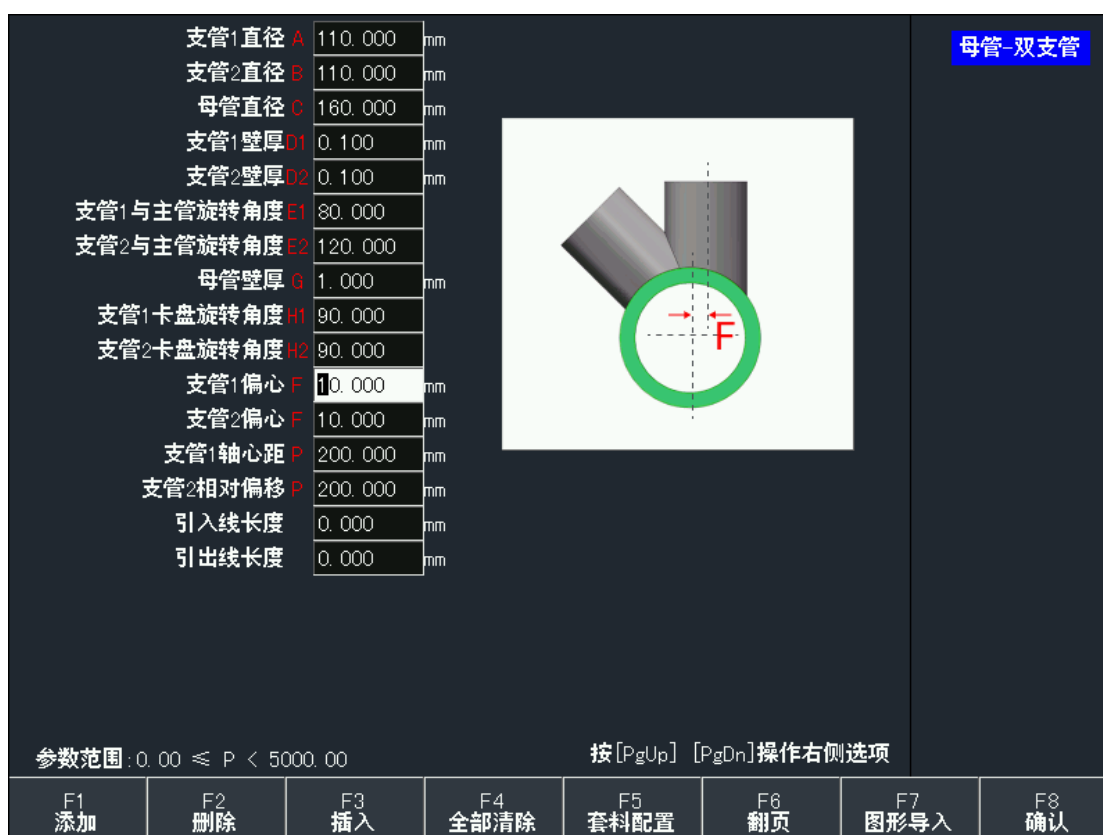
Figure 9.1 6 Main pipe-double branch eccentric
