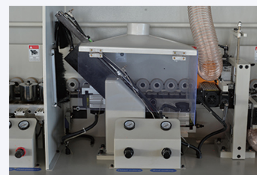
End cutting unit with high speed motor
