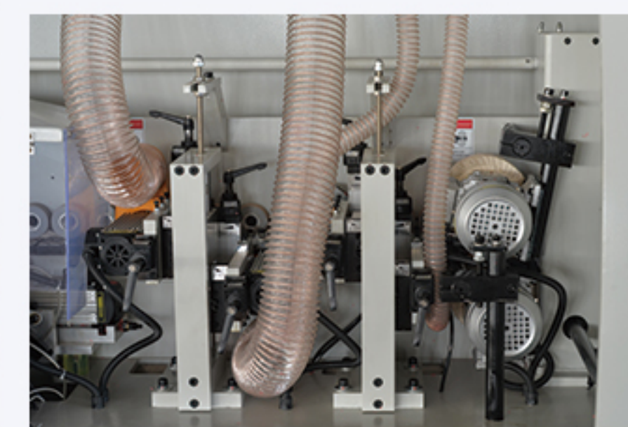
Trimming and buffing units
