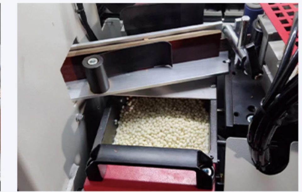
Tefflon-coated glue tank can be replaced easily
