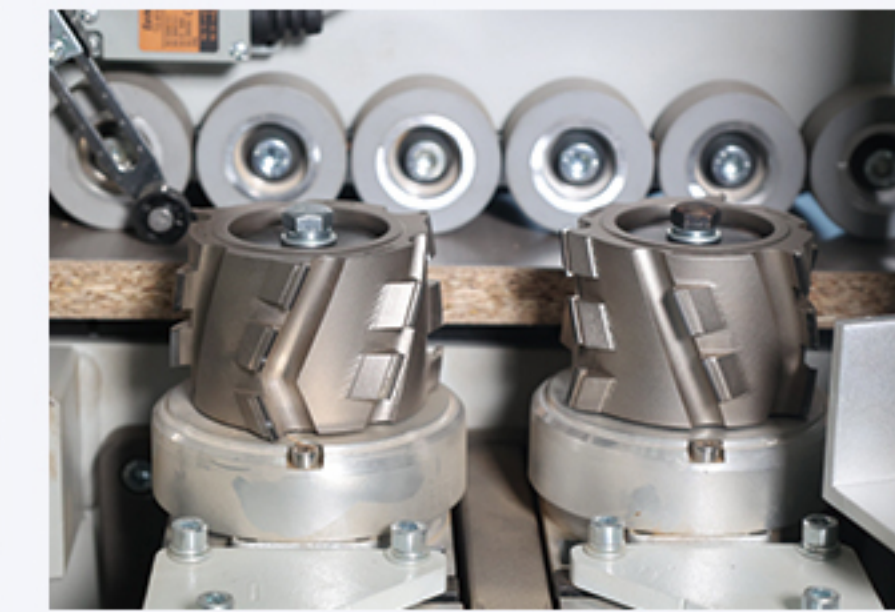
Pre-milling unit with diamond cutters
